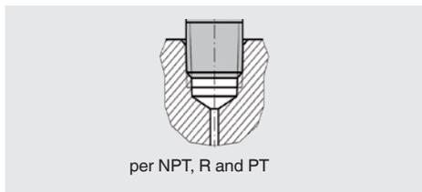
For sealing process connections with tapered threads, the sealing must be made in the threads using additional sealing material - e.g. PTFE tape (EN 837-2).
