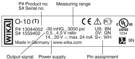
If the serial number becomes illegible due to mechanical damage or overpainting, traceability will no longer be possible.
