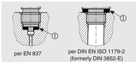
Correct sealing of the process connections with parallel threads at the sealing face ① must be made using suitable flat gaskets, sealing rings or WIKA profile sealings.
