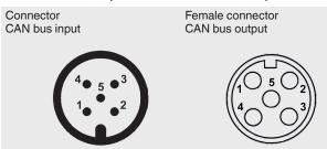
The socket and connector are connected internally.
