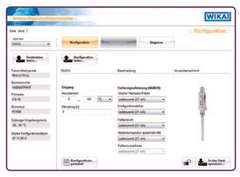
**02** Individually parameterisable for integrated transmitter with free PC configuration software Wikasoft-TT
